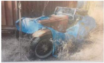
The trip home from Queensland in the trailer managed to shake apart almost all of the timber in the body, so most of my work up to this point has been trying to remake the timber body frame. I have made most of the major timber components & started fitting them together. I am still working up the courage to attack the doors. I have remade rough timber door frames, but at the moment these are standard size timber sections screwed together, awaiting shaping to the correct size & profile
