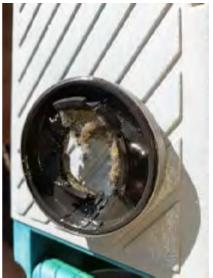
Examination of the inner rubber seal revealed that it had work hardened and aged to be like Bakelite and if it was not for the additional outer felt seal ring the oil probably would have freely flowed out.
