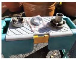
The new seal was half the thickness of the original seal so the rubber sealing surface was not in the same location on the output flange so had a new surface on which to seal. There was no felt ring either in the new seal.
