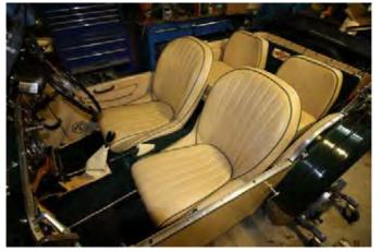
I completed the trimming by edging the carpets myself using a trusty pre war Singer 99k sewing machine. These machines will sew anything you can get under the foot with the right thread and needle. This has proven to be a great tool for any car restoration and well worth the cost.
