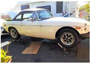
Our final solution was drive the car up my ramps at the front then jack the rear of the car up and place a second set of car ramps under the back wheels. (as shown to the left) After removal of the driveshaft I had my son undo the
