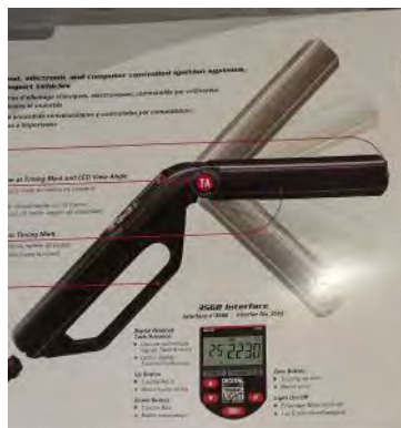
Timing light used to show advance @ specific rpm
